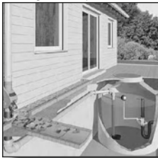
d. rainwater storage and flow regulation systems
