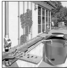
b. rainwater harvesting systems
